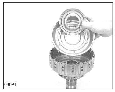
Install new O-ring seals 72.050 and 72.060 on piston B 72.020. Press piston into cylinder B 72.010. Pull O-ring seal 72.100 onto baffle plate 72.080 and press this into the piston.
