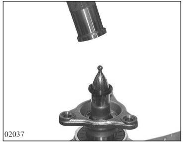
Press shaft sealing ring 14.150 into output flange 14.140 using mandrel 5x46 002 849. Then tighten castellated nut loosely
