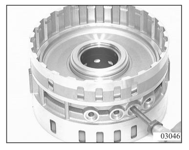
Turn the cylinder around and apply compressed air carefully to the oil feed hole to force out piston C. Pull the 2 O-ring seals off piston C.
