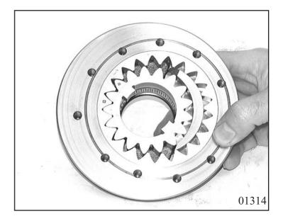
Put 2 rectangular rings 10.040/160 + /170onto the stator shaft 10.040/120. In order to mount the stator shaft on the intermediate plate, these must be positioned towards each other. Follow the procedure stated on the next page.
