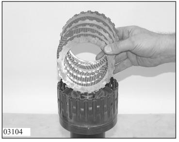
Insert complete clutch pack E. Start with spring disk 71.140, then insert outer disk 71.150 and lined disk 71.160 alternately. Insert final disk 71.150 and secure with snap ring 71.180.
