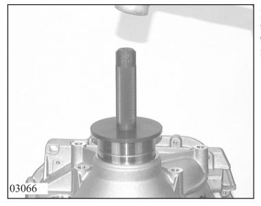
Press needle roller bearing 14.020 into transmission casing using mandrel 5x46 909 346 and supporting ring 5x46 909 347. Secure with snap ring 14.040
