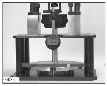
Determine thickness M<sub>D</sub> of the brake D disc cluster as described in Chapter 1.4.0 "Measuring the disk clusters".
