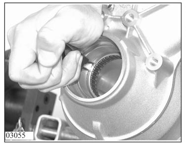
Remove the snap ring with pliers. If necessary, heat the casing around the needle roller bearing with a fan heater to  $70^{\circ}$  C. Turn housing with output side down and remove the needle roller bearing from the transmission casing.
