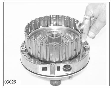
Mount cylinder A on the oil supply unit and force the complete cluster out with compressed air. Take out the planet wheel carrier and cup spring.
