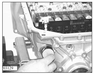
Press in new socket 27.520 with mechatronic screw plug 27.700 attached and secure with retaining clip.
