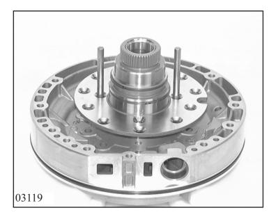
Put the intermediate and centering plates on a supporting fixture and heat up with a hot-air blower to approx. 70 °C. Insert the stator shaft over the locating pins and fasten first with 4 countersunk screws 10.040/150.
