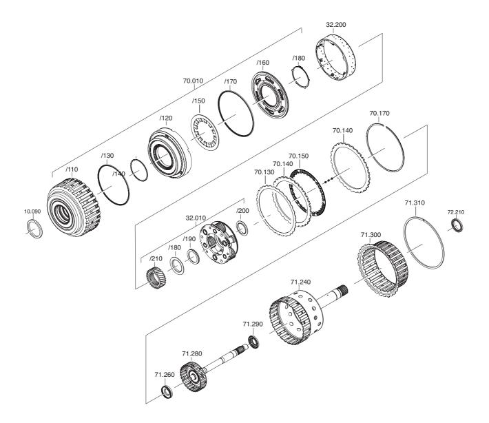
Put 1 new prof. seal ring 70.010/130 and 1 new O-ring seal 70.010/140 onto piston A 70.010/120.
