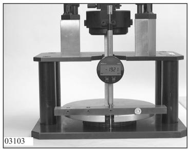
Determining the thickness  $M_E$  of the clutch E disk cluster as described in Chapter 1.4.0 "Measuring the disk clusters".
