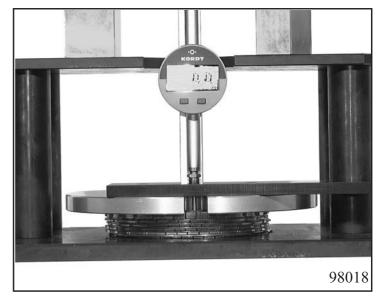
Measure down to the baseplate with the measuring bar.
