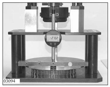
Determine thickness M<sub>B</sub> of the clutch B disk cluster as described in Chapter 1.4.0 "Measuring the disk clusters".
