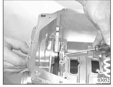
Remove the shaft sealing ring from the transmission casing with a suitable lever. Remove the snap ring with pliers.
