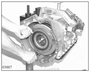
Remove the converter hoop and take out the converter, holding it by the two converter puller handles 5x56 000 090.
