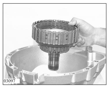
Insert complete clutch B into transmission housing.
