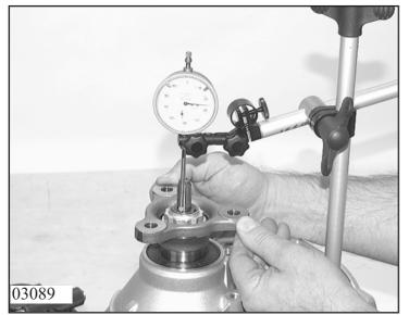
Pull on the flange and read off measurement A. Select a thicker or thinner washer if dimension A is beyond tolerance C.
