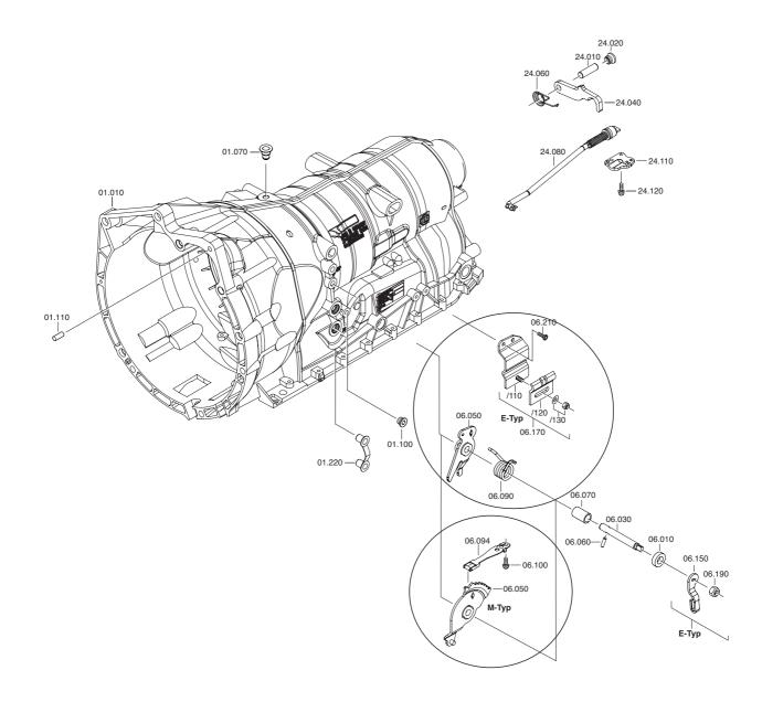
Drive breather 01.070 into transmission casing 01.010 with a plastic-faced hammer.
