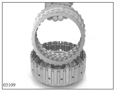
Insert complete clutch pack A. Start with spring disk 70.130, then insert outer disk 70.140 and lined disk 70.150 alternately. Secure the top outer disk 70.140 with snap ring 70.170.
