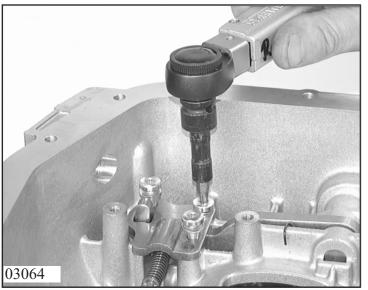
Press down ratchet and fasten guide plate 24.110 with 3 Torx screws 24.120.
