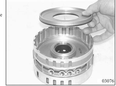
Insert cup spring C 75.070. Press down cup spring C in the mandrel press with assembly bracket 5x46 909 247 and secure with devided snap ring 75.080.
