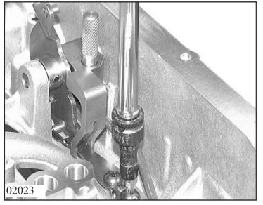
Detent spring with centering device Align 5x46 002 292 and in this position, tighten the detent spring. Tighten the screw on the output side first.
