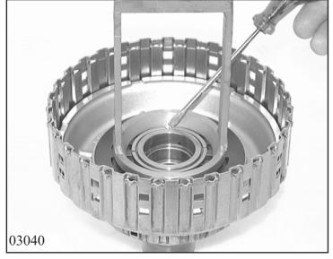
Using assembly hoop 5x46 909 248, press cup spring B out in the arbor press. Remove the split retaining ring and take out the divided cup spring.
