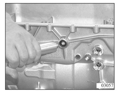
Insert new screw plug 01.100. Press in 2 transport plugs 01.220 by hand.
