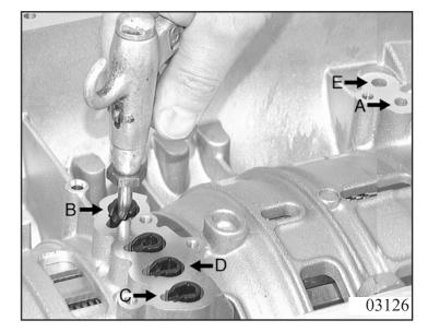
Insert sealing element 27.460 into the transmission casing.
