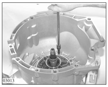
Turn the transmission by 90 degrees. Remove the complete oil supply system by unscrewing the 11 torx screws and taking them out complete with the Usit rings.
