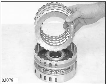
Insert complete clutch pack C into cylinder CD, starting with spring disk 75.100. Then insert an outer disk 75.140 and a lined disk 75.120 alternately. Secure the top outer disk 75.150 with snap ring 75.180.
