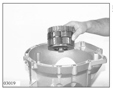
Remove sun wheel 2 with angle plate. Take out the planet wheel carrier.
