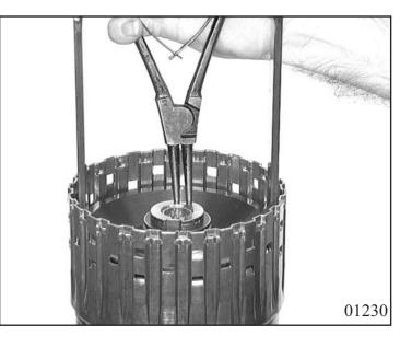
Plug one of the two oil feed holes and force piston E out with compressed air. Pull off the two O-ring seals.
