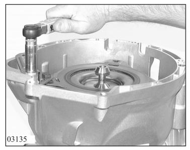
Remove converter handles. Turn transmission by 90° Screw on converter retaining bracket 97.010 with 1 screw 97.020 on gearboxhousing and 1 srew on converter 97.030.
