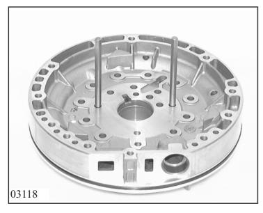
Place intermediate plate 10.040/110 onto centering plate 10.040/130 and position. Srew 2 locating pins 5x46 001 007 into centering plate.
