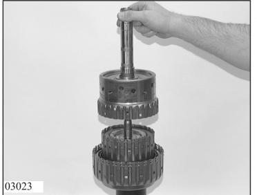
Take out inner disk carrier A and lever the needle roller thrust bearing out of the intermediate shaft, using a long scriber as a tool.
