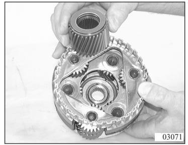
Turn transmission with converter bell upwards.
