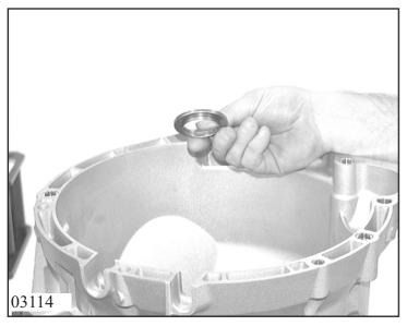
Place axial needle roller cage 72.210 with angle disk facing down on the hub of cylinder B.
