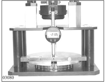
Determine thickness M<sub>C</sub> of the brake C disk cluster as described in Chapter 1.4.0 "Measuring the disk clusters".
