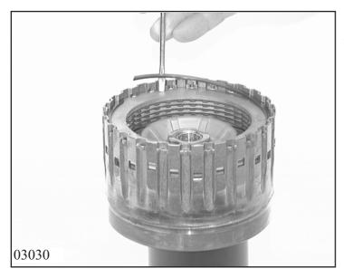
Take out the snap ring for clutch E and remove the complete clutch E disk set.
