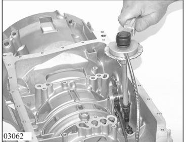
After this, use auxiliary tool 5w04 000 583 to turn farther by the amount of angular offset. Remove the centering device. Shift the selector shaft through all positions, then remove.
