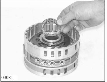
Turn cylinder CD and clip axial needle bearing 42.290 into position at the cylinder web.
