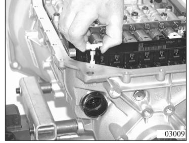
Unscrew and remove the **large-headed** screws (M6) and lift off the complete Mechatronic assembly.
