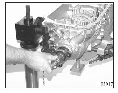
Turn the transmission by 90 degrees and lever out the snap ring from the casing with a suitable screwdriver or take it out with snap ring pliers. Lift out clutch CD.
