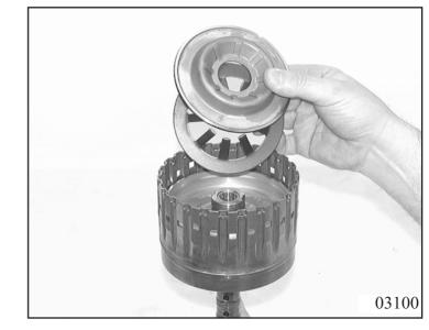
Insert assembly adapter 5x46 003 343. Put new snap ring 71.100 on top. Press pipe with snap ring and cup spring down in the mandrel press until the snap ring engages in the slot.
