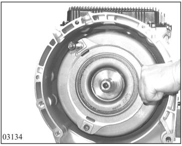
Move converter back and forward until the pump drive pins engage.
