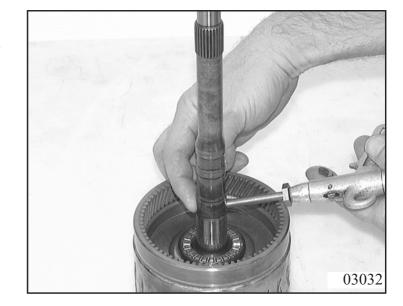
Pull the three rectangular-section rings off the input shaft.
