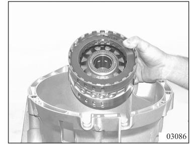
Secure with snap ring 73.210. Use driving-in tool 5x46 001 930 to drive the snap ring into the housing groove all round.
