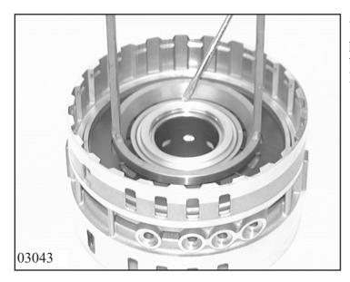
Using assembly hoop 5x46 909 247, press cup spring C out in the arbor press; take out the split retaining ring. Remove the devided cup spring
