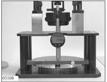
Determine thickness  $M_A$  of the clutch A disk cluster as described in Chapter 1.4.0 "Measuring the disk clusters".
