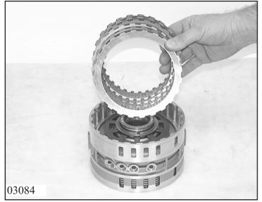
Insert complete clutch pack D into cylinder CD, starting with spring clutch disk 73.150 and then insert lined disk 73.170 and external disk 73.216 alternately. Secure final disk 73.180 with snap ring 73.190.
