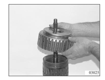
**Caution:** Input shaft is splined to clutch E.
