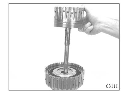
Align discs of clutches A and E and insert intermediate shaft 71.280 by turning slightly.
