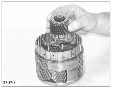
Using a suitable tool, separate the sun wheel from the bearing in the planet wheel carrier; take another sun wheel 3 out of the planet wheel carrier and unclip the bearing from sun wheel 3. Remove the bearing from the planet wheel carrier.
