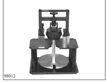
Tighten the 4 knurled screws 5p01 000 329 to secure the adjusting fixture firmly with the height measuring fixtures by way of the spacers.
