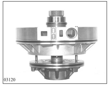
Screw locating pins 5x46 001 007 into pump. Mount complete pump over stator shaft, remove locating pins and tighten with 11 machine screws 10.050.
