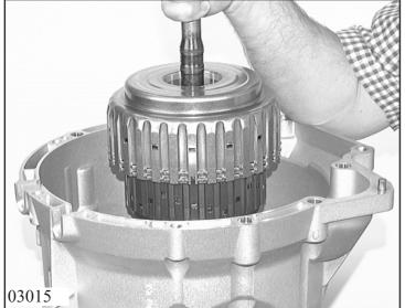
Take out the shim washer. Remove the turret (input with clutches A and E).
