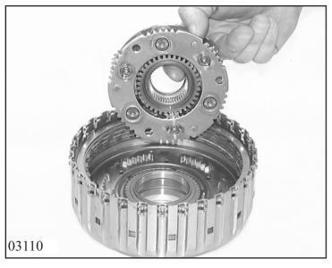
Insert sun wheel 32.010/210 with axial needle cage facing the inside of the planet gear set 32.010.
