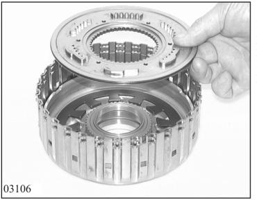
Insert cup spring 70.010/150. Put prof. seal ring 70.010/170 onto baffle plate 70.010/160 and insert the baffle plate into the cylinder. Press the cup spring down in the mandrel press with assembly bracket 5x46 909 247 and secure with K-ring 70.010/180.
