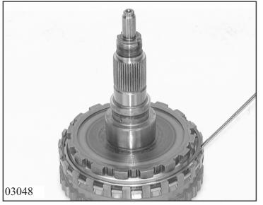
Separate the output shaft from the ring gear by levering out the snap ring.
