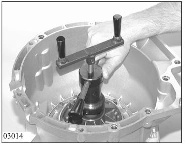
Press out the oil supply unit with lifter 5x46 002 009 and lift it off.
