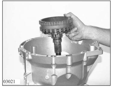
Take out the ring gear with output shaft. Unclip the bearing from the planet wheel carrier hub.
