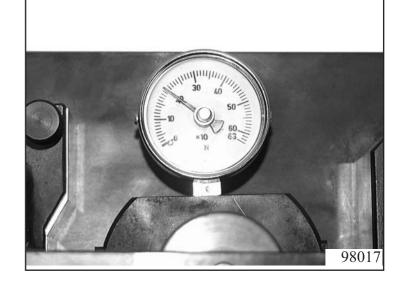
Next, place measuring bar 5p01 000 330 on the measuring plate, place the measuring foot of the dial gauge in the groove of the measuring plate on the upper disk of the disk cluster, and set the dial gauge to "0".
