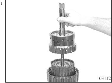
Insert inner disk carrier B 71.300 into cylinder A and secure with snap ring 71.310.
