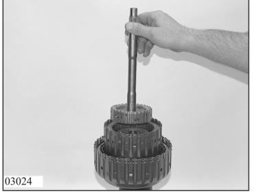
Lift off the intermediate shaft with inner disk carrier B. Lever out the needle roller thrust bearing.
