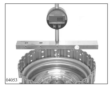
Determine thickness M<sub>B</sub> of clutch B clutch pack according to Chapter 1.4.0 Measuring clutch pack.
