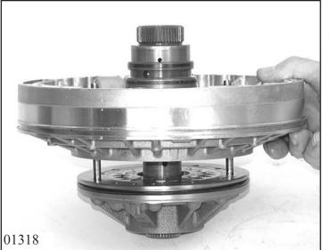
Screw locating pins 5x46 001 007 into pump. Mount complete pump over stator shaft, remove locating pins and tighten down with 11 machine screws 10.050.
