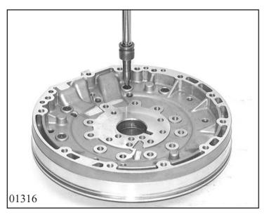
Place intermediate plate 10.040/110 on centering plate 10.040/130 and hold it in position with 4 screws 10.040/180, but without tightening.
