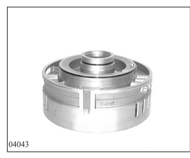
Drive 2 shaft keys 75.010/140 in centrally at cylinder CD 75.010, using a plastic hammer. Pull 1 O-ring seal 73.080 onto piston D 73.010 and 2 O-ring seals 73.020 + 73.030 onto cylinder CD 75.010.
