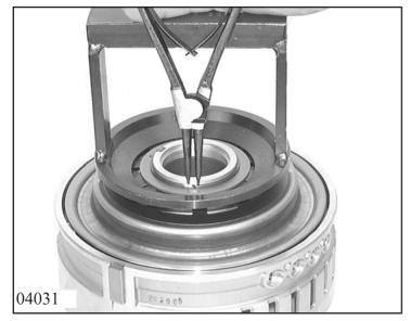
Turn the cylinder around and clip out the bearing. Press down cup spring D in the mandrel press with assembly bracket 5x46 000 221; take out snap ring and stop washer and remove cup spring.
