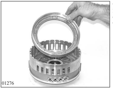
Turn cylinder CD by 180°. Put 2 O-ring seals 75.040 and 75.050 onto piston C 75.030 and press it into the cylinder.
