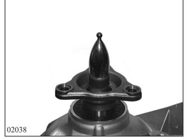
Press shaft sealing ring 14.150 into output flange 14.140 using mandrel 5x46 002 849.
