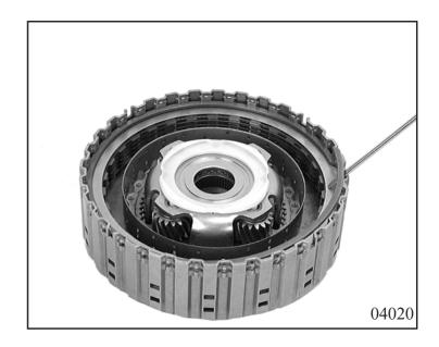
Lever snap ring out of planet carrier and take planet carrier out of cylinder A. Withdraw snap ring and sun gear from planet carrier and lever out axial needle roller bearing cage.
