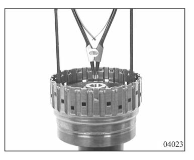
Cover one of the two oil guide bores and press out piston E with compressed air. Pull off the two O-ring seals.
