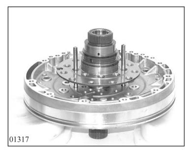
Put the intermediate and centering plates on a supporting fixture and heat up with a hot-air blower to approx. 70 °C. Screw 2 locating bolts 5x46 001 007 into the centering plate. Insert the stator shaft over the locating pins and fasten first with countersunk screws 10.040/150. Remove the locating pins, insert the remaining two countersunk screws and tighten the 4 screws previously screwed in.
