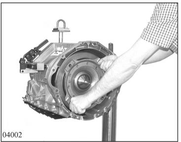
Remove converter bracket and take out converter using the two converter pull-out handles 5x56 000 090.
