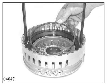
Insert cup spring C 75.070 and retaining ring 75.080.
