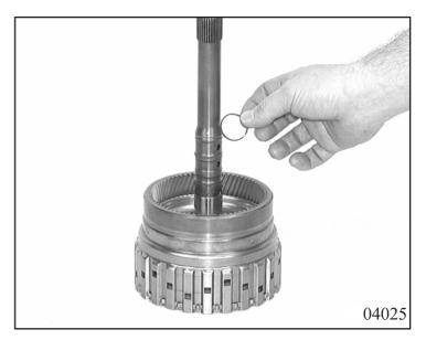
**Note!** Unclip needle roller bearing if defective.
