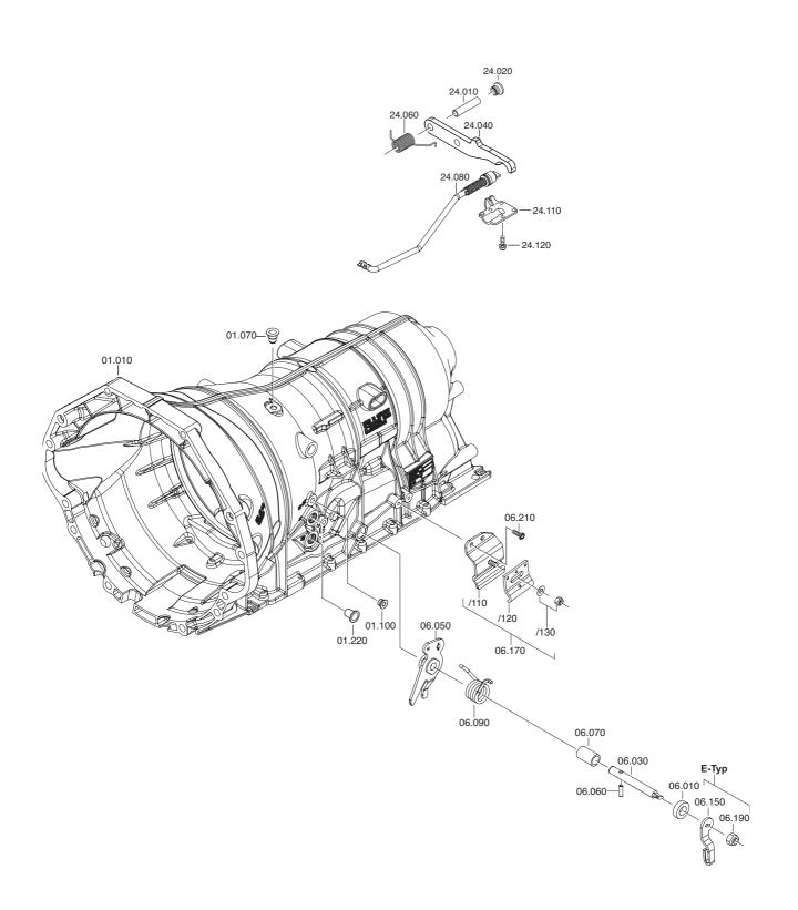
Drive breather 01.070 into transmission casing 01.010 with a plastic-faced hammer.
