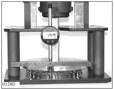
Determine thickness M<sub>C</sub> of brake C clutch pack according to Chapter 1.4.0 Measuring clutch pack.
