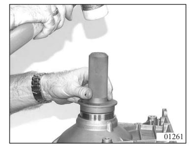
Press shaft sealing ring 14.110 into transmission casing using mandrel 5x46 002 567.
