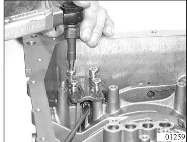
Attach emergency release angle 06.170 with two Torx screws 06.210 Fasten lever 06.150 facing the oil pan side with nut 06.190.
