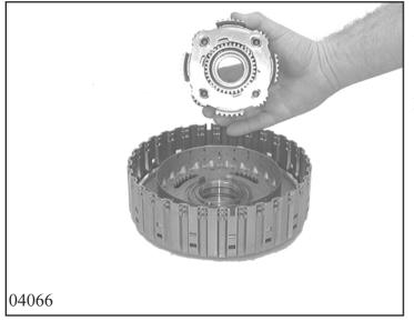
Insert bearing in sun wheel. Insert sun wheel 32.010/210 and snap ring 32.010/ 220 into planetary gear set 32.010. Engage complete planetary gear set in position on cylinder A.
