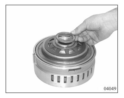
Insert complete clutch pack D into housing, starting with final disk 73.260, then insert lined disk 73.250 and external disk 73.240 alternately. Complete with spring disk 73.230.
