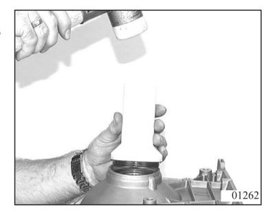
Mount ring gear 42.170 with snap ring 42.180 on output shaft 42.190. Secure compensating washer 14.050 previously removed with grease to the output shaft. Turn the transmission by 90°.
