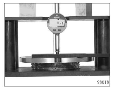
Now use the measuring bar to measure down to the base plate.
