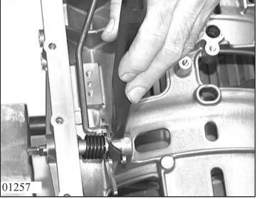
Drive in new dowel pin 06.060 with striker pin 5x46 000 291 or an appropriate mandrel in the correct position.
