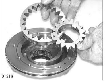
Pull off O-ring seal. The pump can be dismantled by taking out the impeller and ring gear.
