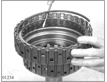
Turn cylinder by 180°, take out clutch B snap ring and take out the complete clutch pack.
