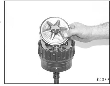
Insert angular plate 71.094 with groove facing upwards.
