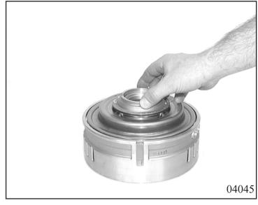
Insert cup spring 73.120. Press cup spring down in the mandrel press with assembly bracket 5x46 000 221 and secure with snap ring and stop washer 73.130.
