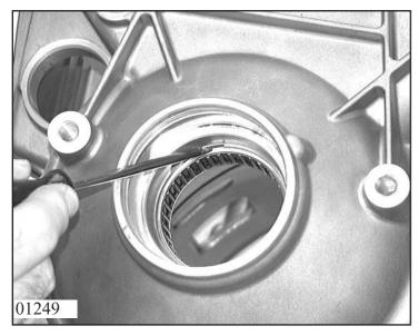
Press needle roller bearing 14.020 into transmission casing using mandrel 5x46 002 559.
