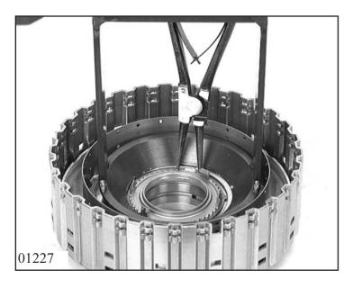
Press down cup spring in the mandrel press with assembly bracket 5x46 002 566 and remove snap ring with suitable pliers. Take out baffle plate and cup spring.
