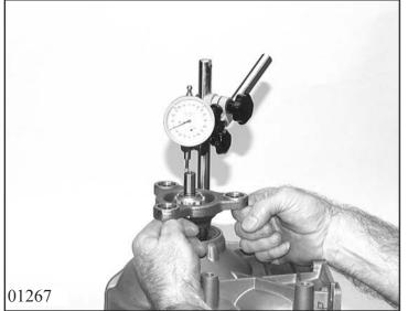
Pull on flange and read off value **A**. Select a thinner or thicker disk if value A is outside tolerance C.
