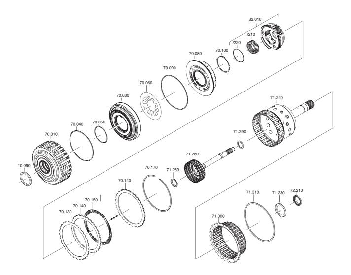
Put 2 O-ring seals 70.040 + 70.050 onto piston A 70.030. Press piston A into cylinder A 70.010.
