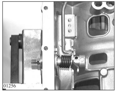
Insert parking or detent disk with connecting rod into transmission casing and push in selector shaft 06.030 through sleeve 06.070, spring 06.090 and detent disk. Put in spring.
