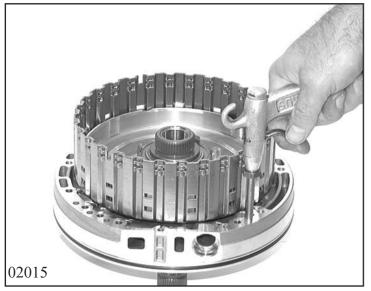
Place cylinder A on top of the oil supply and press out piston with compressed air. Pull 2 O-ring seals off piston A. Remove cylinder A from oil supply
