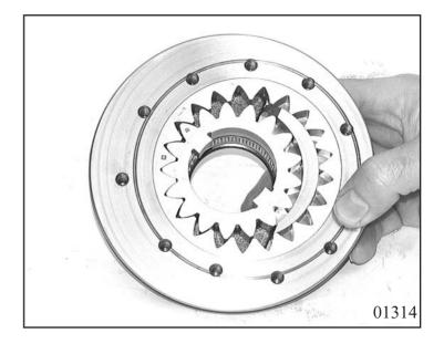
Put 2 cylindrical rings 10.040/160 + /170onto the stator shaft 10.040/120. So that the stator shaft can be mounted on the intermediate plate, these must be positioned towards each other. Follow the procedure stated on the next page.
