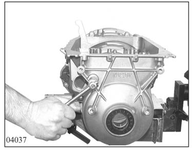
Remove screw plug with sealing ring.
