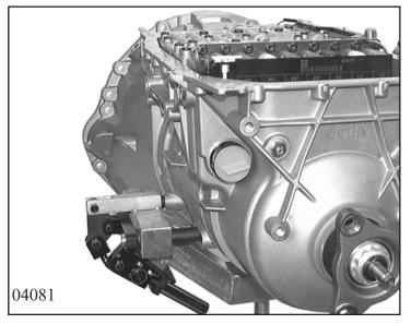
Press in new socket 27.520 **•** with mechatronics screw plug 27.700 attached **•** and secure with retaining clip. J
