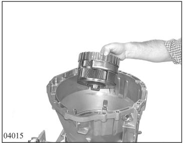
Take out the angle plate and sun gear. Remove planet carrier. Remove clutch pack D from transmission casing.
