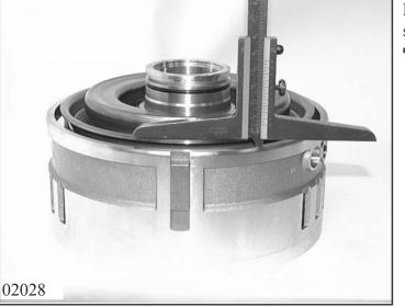
Measure down from piston to cylinder support area CD and read off dimension  $\Rightarrow M_{DB}$ .
