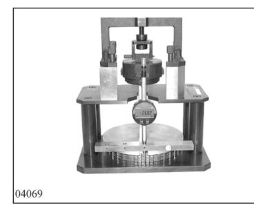
Determine thickness  $M_A$  of clutch A clutch pack according to Chapter 1.4.0 Measuring clutch pack.
