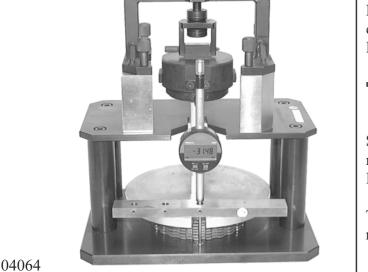
Determine thickness  $M_E$  of clutch E clutch pack according to Chapter 1.4.0 Measuring clutch pack.
