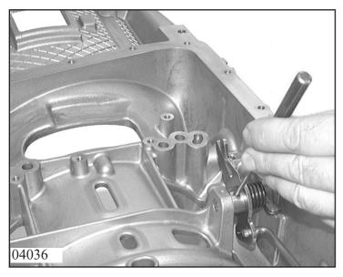
Drive clamping sleeve out of parking disk with a suitable mandrel and pull out selector shaft. Remove sleeve and spring.
