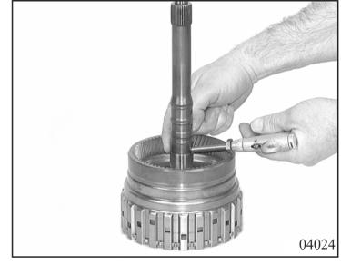
Pull the O-ring seal and 3 rectangularsection rings off the drive shaft.
