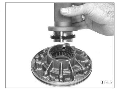
Put on new O-ring seal 10.020. Lubricate the pump wheel and internal ring gear lightly before assembly. Then assemble the pump in such a way that one marking is visible both on the pump wheel and the internal ring gear.
