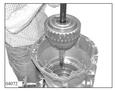
Place assembly tool 5x46 002 563 over the innput shaft and lock with pin. Align disks of clutch B, insert turret and turning it in both directions until the disks engage fully in disk carrier B.
