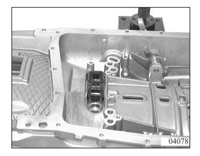
Check all clutches / brakes for proper function by supplying compressed air to the marked bores (see picture alongside) Place mechatronics.
