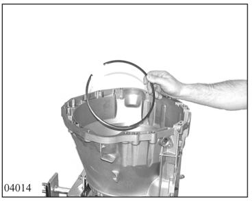
Turn transmission by 90° and lever snap ring out of casing with a screwdriver or take it out with snap ring pliers. Lift off clutch C. Remove angle disk
