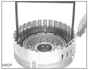
Press down cup spring C in the mandrel press with assembly bracket 5x46 909 303, lever out the snap ring and remove the cup spring.
