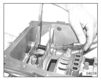
Remove the shaft sealing ring from the transmission casing with a suitable lever.
