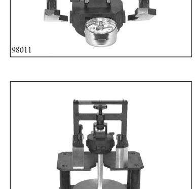
Fasten it with 4 knurled screws to the measuring fixture using the intermediate pieces.
