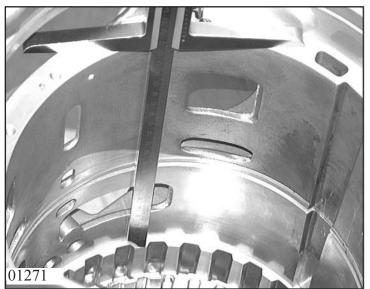
Place measuring base on cylinder support area CD in the housing and read off dimension ▷ W<sub>DB</sub>.
