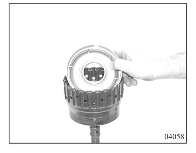
Put new O-ring seal 71.090 onto baffle plate 71.080. Insert cup spring 71.060 into cylinder E with the projections facing downwards and press in the baffle plate.
