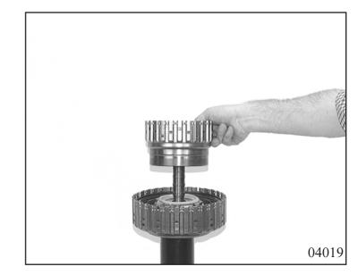
Note: Drive shaft is splined to clutch E.
