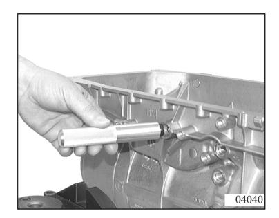
Insert new screw plug 01.100. Press in transport plugs 01.220 by hand.
