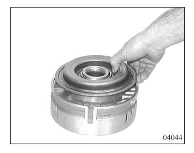
Put 1 O-ring seal 73.070 onto baffle plate D 73.060 and press it into piston D.
