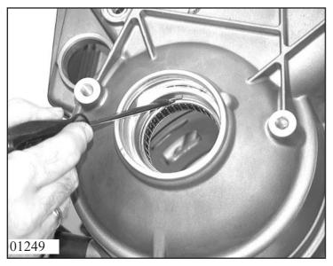
Remove the snap ring with pliers. If necessary, heat the casing around the needle roller bearing with a fan heater to 70° C. Turn housing with output side down and remove the needle roller bearing from the transmission casing.
