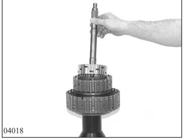
Lift off intermediate shaft with internal disk carrier E. Lever out axial needle roller bearing.
