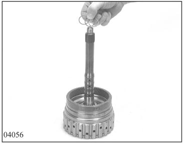
Put 3 new rectangular-section rings 71.190 onto cylinder E 71.010 with input shaft.
