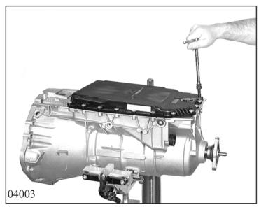
Turn transmission by 180°. Unscrew 21 machine screws holding the oil pan, remove it and pull off the O-ring seal and gasket.
