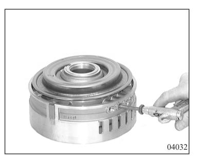
Press out piston C with the air sensor. Pull 2 O-ring off piston C.
