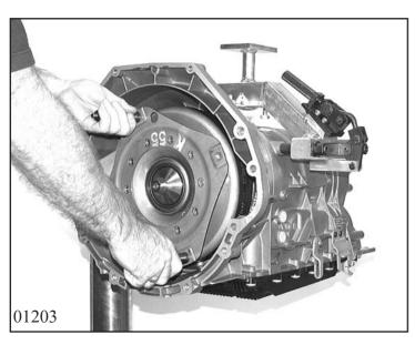
Remove converter bracket and take out converter
