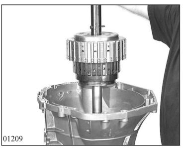
Take out the shim washer. Remove turret (input with clutches A and E).
