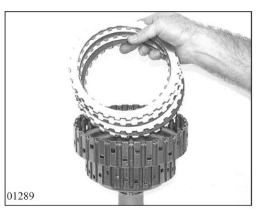
Determine thickness  $\mathbf{M_B}$  of clutch B clutch pack according to Chapter 1.4.0 Measuring clutch pack.
