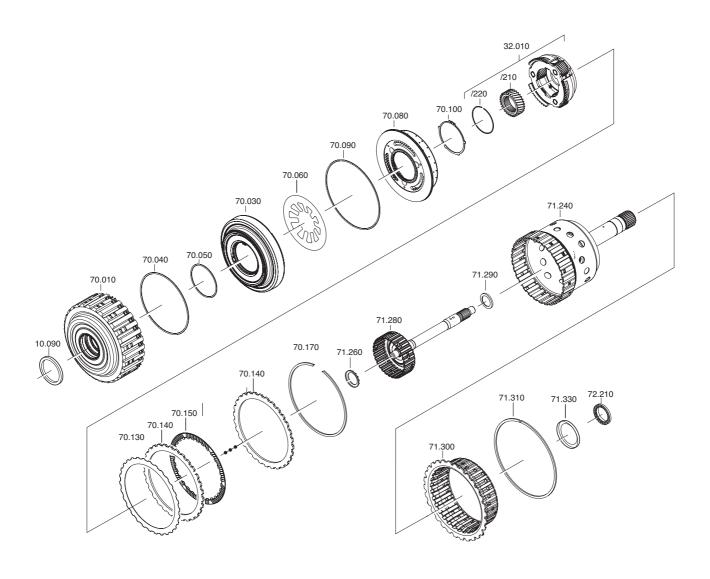
Pull 2 O-ring seals 70.040 + 70.050 onto piston A 70.030.
