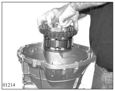
Take out the angle plate and sun gear. Remove planet carrier with complete clutch pack D.
