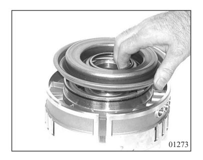
Pull 1 O-ring seal 73.070 onto baffle plate D 73.060 and press it into piston D. Press the air baffle plate down and secure with split retaining ring 73.100+73.110.
