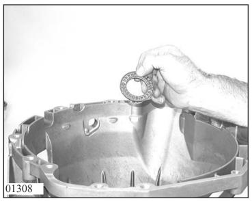
Place axial needle roller cage 72.210 on the hub of cylinder B.
