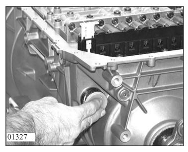
Press in new socket 27.520 **u** with mechatronics screw plug 27.700 attached **u** and secure with retaining clip. J
