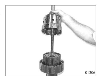
Insert inner disk carrier B 71.300 into cylinder A and secure with snap ring 71.310.
