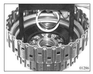
Insert complete clutch pack B, starting with spring disk 72.130. Then insert outer disk 72.140 and lined disk 72.150 alternately.
