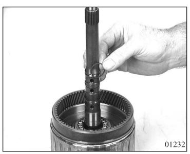
Note! Unclip needle roller bearing if defective.
