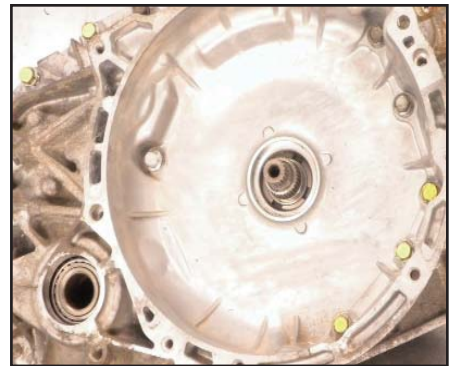
Remove bell housing bolts.
