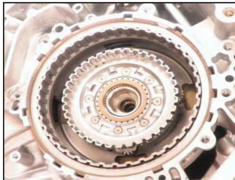
Remove planetary assembly
