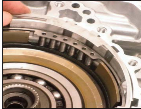
Install reverse clutch, return springs and retainer plate
