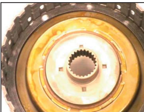
Install cushion plate dish down
