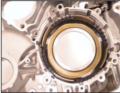
Install reverse clutch piston
