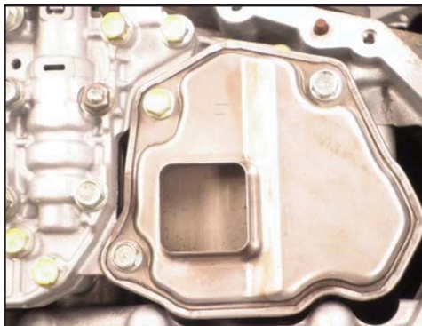
Remove the filter
