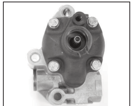
Torque cover bolts 19 Ft. Lbs. (26Nm)
