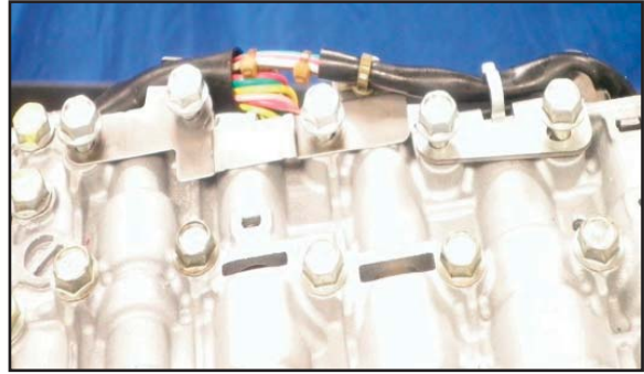
Install wiring harness bracket
