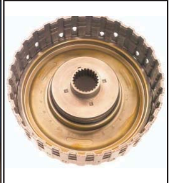
Remove forward clutch balance piston
