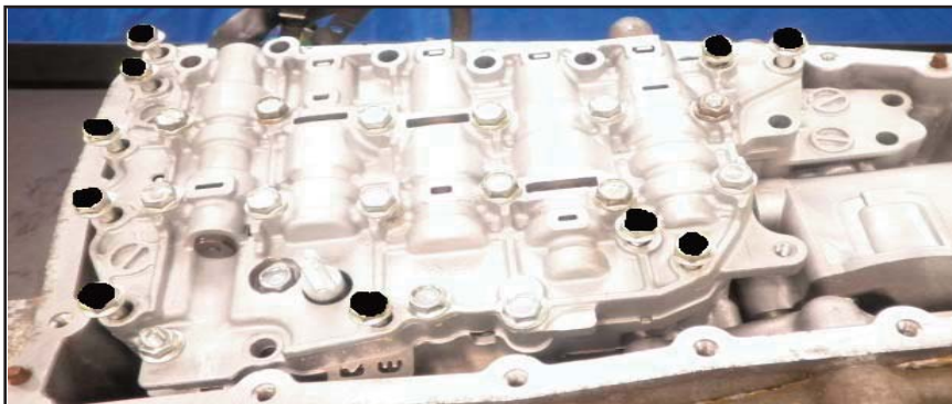
Remove marked bolts to remove valve body.
