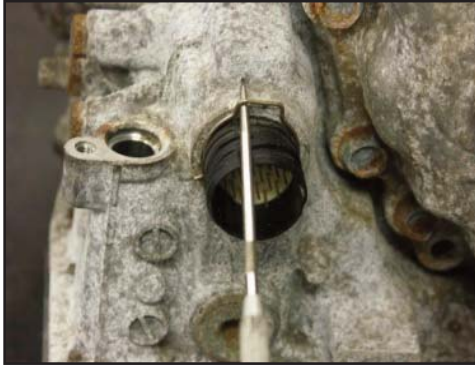
Remove clip holding in case center
