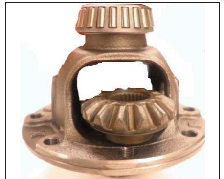
Remove both side gears and washers
