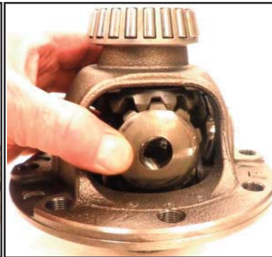
Install the spider gears and washers
