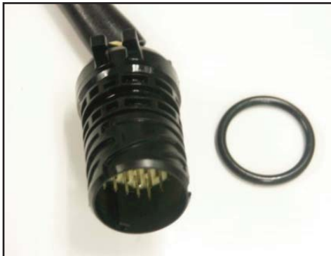
Install case connector into case
