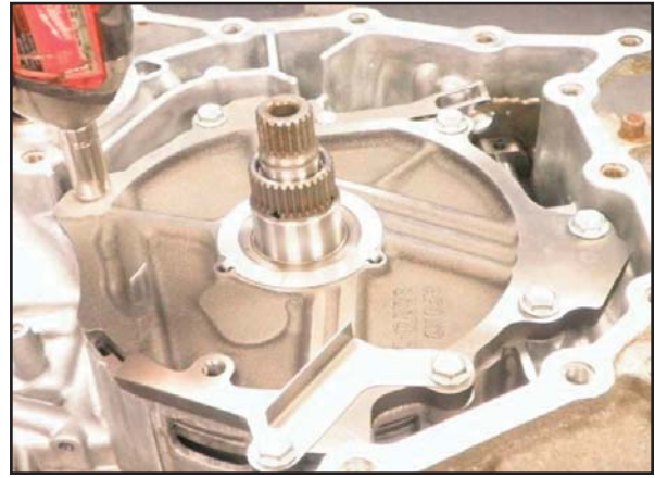
Remove stator support.
