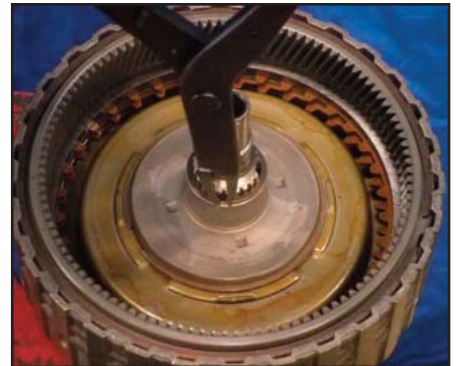
Install input shaft and snap ring
