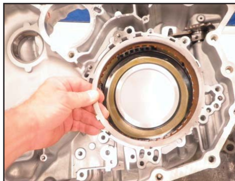
Install the reverse pressure
