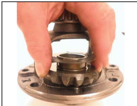
Remove both side gears and washers
