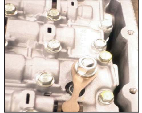
Remove the manual lever
