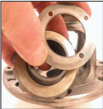
Install both side gears and washers.
