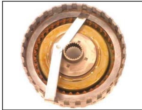
Check clutch pack clearance .047-.059 (1.2-1.5 Nm)
