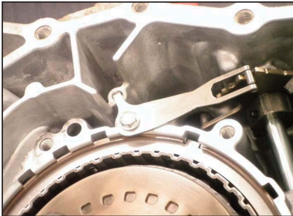
Remove detent spring
