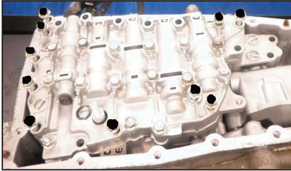
Install valve body and filter bracket
