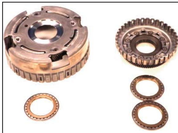
Inspect teeth, pinions for excessive play and pinion washers for wear.
