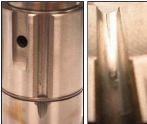
Compress balance piston
