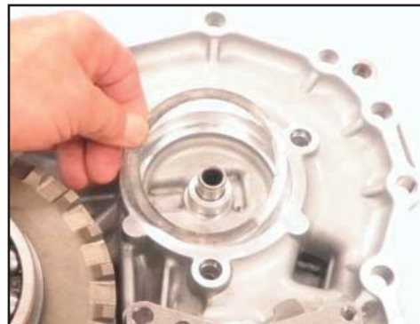
Remove the driven pulley shim
