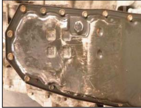
Remove the oil pan
