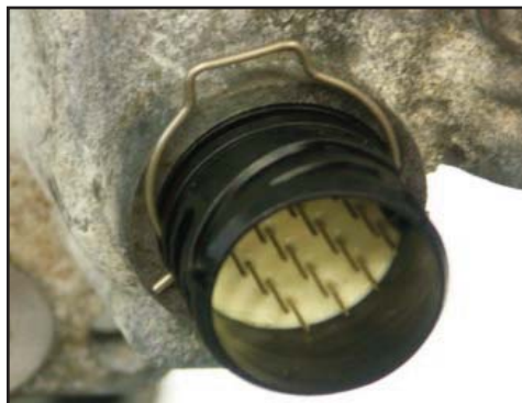
Install case connector clip
