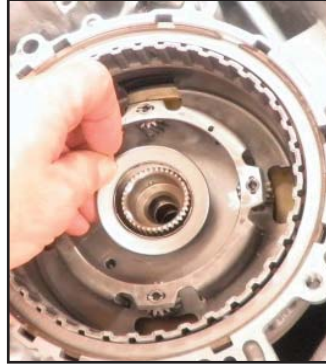
Install torrington bearing and sun gear into planet carrier
