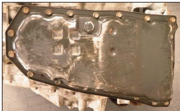
Install oil pan and gasket. Tighten bolts to 70 In. Lbs. (8Nm)
