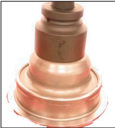
Compress balance piston
