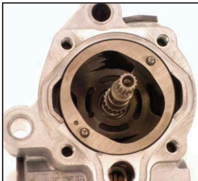
Install pump shaft
