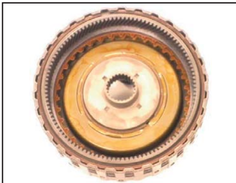
Install ring gear and upper snap ring
