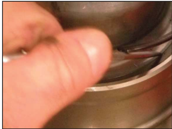
Remove piston retainer snap ring
