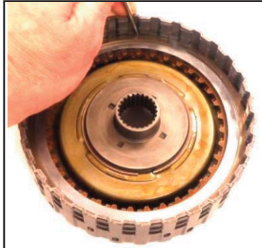
Remove the snap ring, pressure plate clutches and steels
