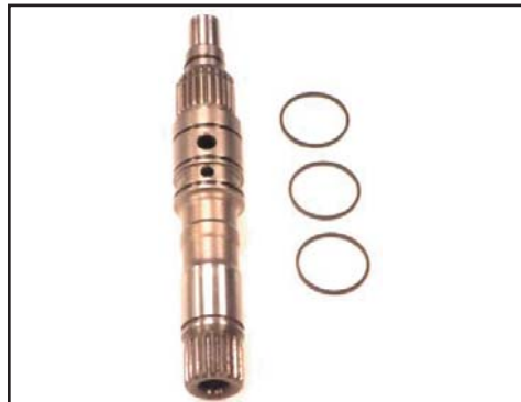
Replace input shaft sealing rings
