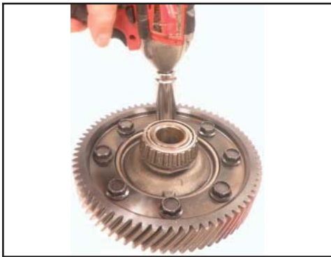
Remove ring gear
