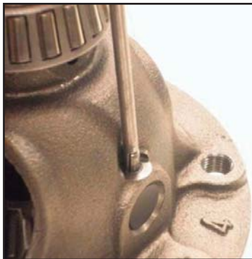
Install roll pin
