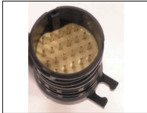
Tang on case connector faces down towards recessed in case
