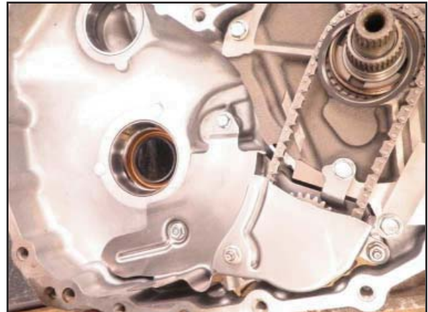
Remove o-ring, selective washer and upper baffle
