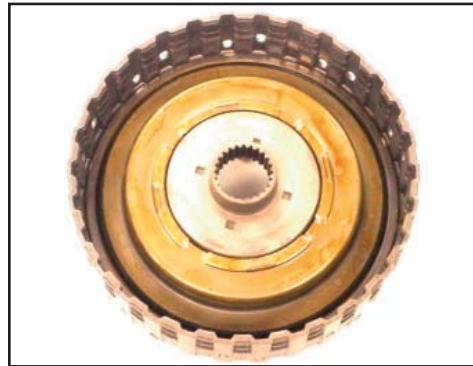
Install balance piston
