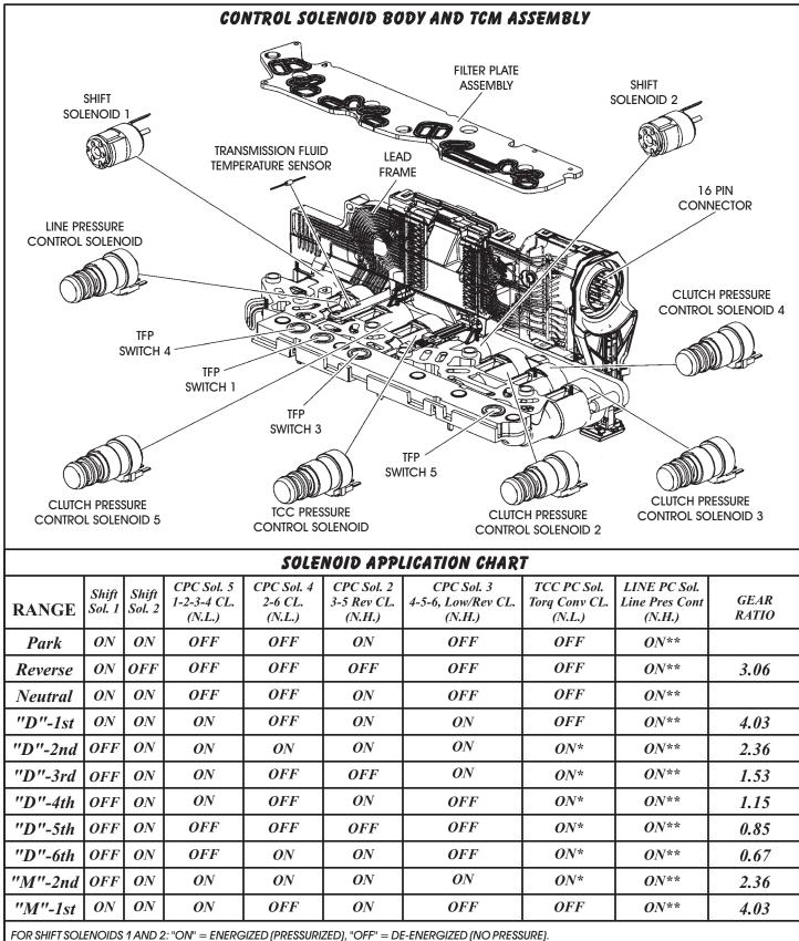
FOR SPILE SOLENOIDS 'I AND Z. ON = ENERGIZED (PRESSURIZED), OFF = DE-ENERGIZED (NO PRESSURE). FOR CPC SOLENOIDS 2, 3: "ON" = NO PRESSURE, "OFF" = PRESSURIZED. FOR CPC SOLENOIDS 4, 5: "ON = PRESSURIZED, "OFF" = NO PRESSURE.
