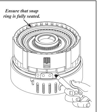
Apply air pressure, regulated to 60 psi, to verify proper installation of all Low/Reverse clutch components, as there are NO selectives. Copyright © 2007 ATSG
