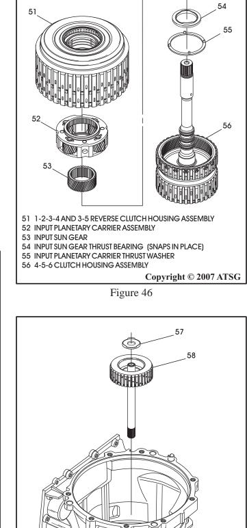
57 4-5-6 CLUTCH HUB TO TURBINE SHAFT THRUST BEARING
