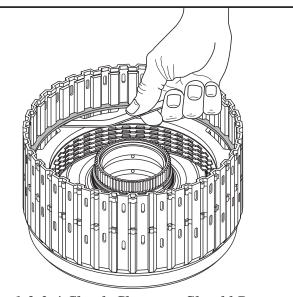
1-2-3-4 Clutch Clearance Should Be 1.53-1.99mm (.060" - .078")
